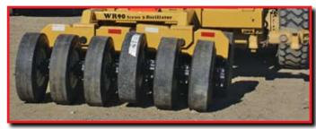
The Hydraulic Side-Shift is a separate module and it can be purchased with the Walk 'n' Roll or added later. The Side Shift is available in 24" or 36". The unit shown is a 36" side shift with receivers to fit a rear ripper. It is also available with quick attach brackets for the ripper or a lift assembly.
