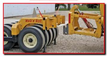
The Heavy Duty Lift Assembly attaches to the motor grader like a factory rear ripper. It uses the same bolt pattern so there is no welding or holes to drill to mount the lift assembly. The lift assembly requires an extra valve and hydraulics to the rear of the motor grader.
